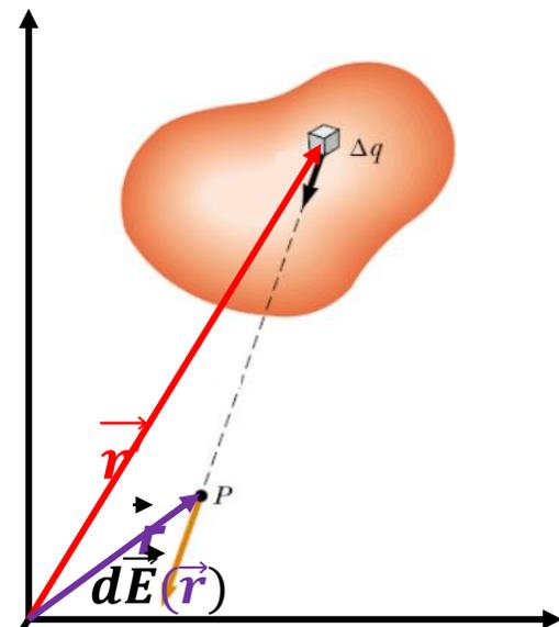
$$E_x(x_0, y_0, z_0) = \frac{1}{4\pi\epsilon_0} \iiint \frac{\rho(x', y', z')(x - x') dx' dy' dz'}{[(x - x')^2 + (y - y')^2 + (z - z')^2]^{3/2}}$$
