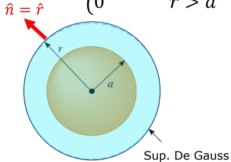
$$\begin{aligned} \Phi &= \oiint \vec{E}(\vec{r}) \cdot d\vec{S} = \oiint E(r) \hat{r} \cdot \hat{r} dS \\ &= E(r) \iint r^2 \sin\theta d\theta d\varphi = E(r) 4\pi r^2 \end{aligned}$$
