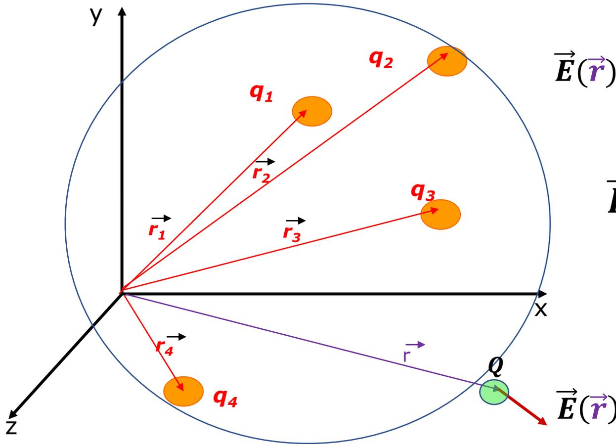
$$\vec{E}(\vec{r}) = \vec{E}_1(\vec{r}) + \vec{E}_2(\vec{r}) + \vec{E}_3(\vec{r}) + \vec{E}_4(\vec{r})$$
